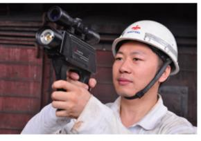
测炉温 Measuring the temperature of the furnace
